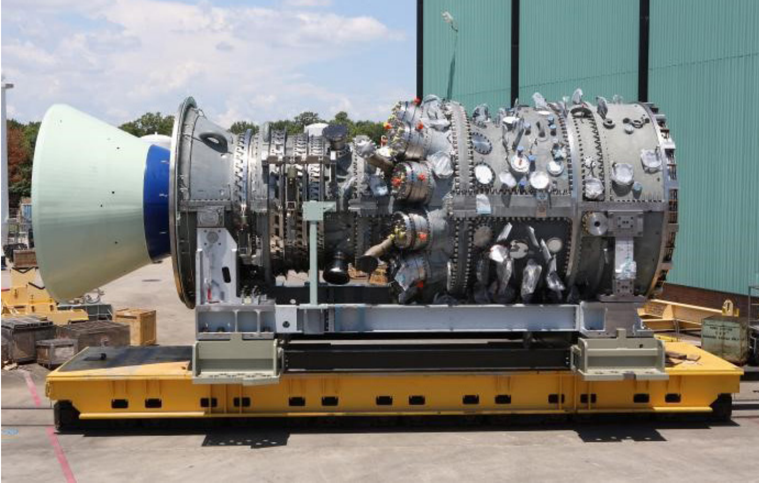
New high-efficiency turbine designs, such as this General Electric 7HA.02 (formerly frame 7) gas turbine, expose turbine oils to higher temperatures and flows compared to older turbines. Source: Oak Ridge National Laboratory
