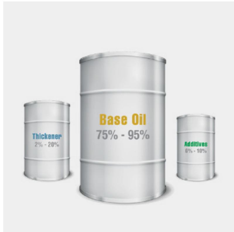
Figure 1. The three primary constituents of an industrial grease. Source: Phillips 66
